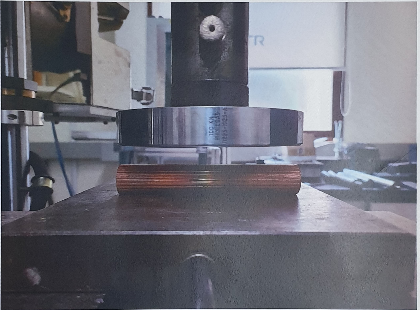
Compression load test
